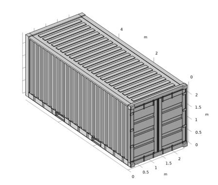
Figure 26 - Geometry of a 20 foot container (snapshot from DBIs model in COMSOL multiphysics)
