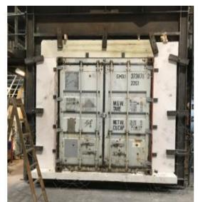
Figure 16 – Door mounted on furnace
