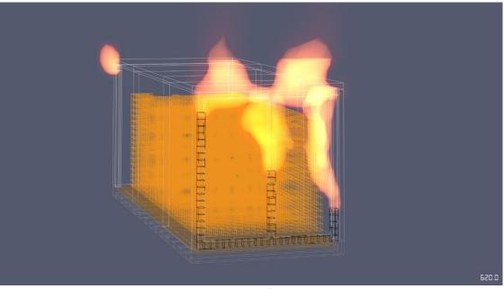
Figure 41: Burn away of the door gasket
