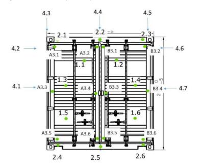
Figure 18 – Thermocouple placement on door
