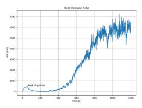
Figure 46: Total HRR during the simulation time
