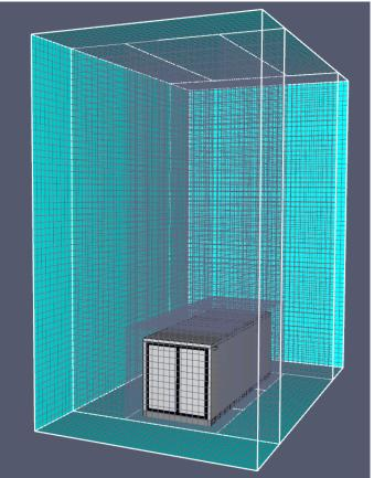
Figure 28: Container and the computational domain Figure 29 shows the door section of the container and the door gasket.
