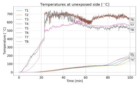
Figure 21 – Temperature reading from the mobile furnace test
