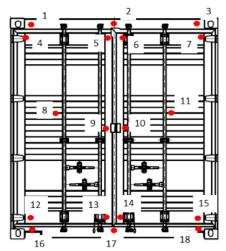
Figure 19 – deflection measurement point placement
