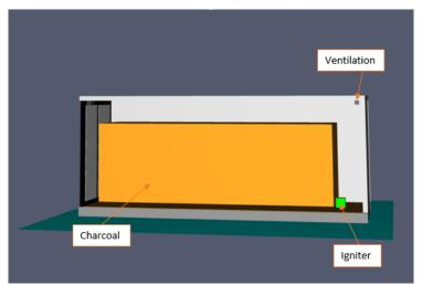
Figure 31: Container content and igniter
