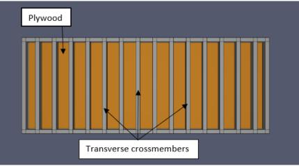
Figure 30: Container understructure
