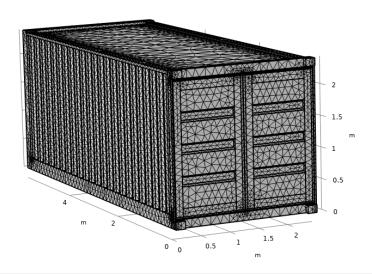
Figure 27 - Meshed container using shell and solid 3D elements
